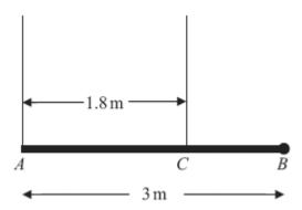
A pole AB has length 3 m and weight W newtons. The pole is held in a horizontal position in equilibrium by two vertical ropes attached to the pole at the points A and C where AC = 1.8 m, as shown in the diagram above. A load of weight 20 N is attached to the rod at B. The pole is modelled as a uniform rod, the ropes as light inextensible strings and the load as a particle.
